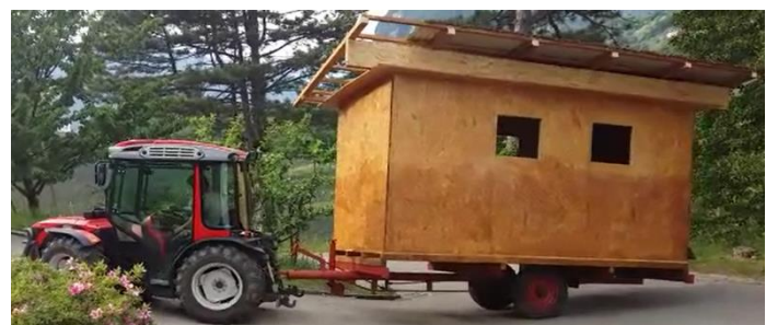
Figure 9: Unfinished mobile broiler barn during the first driving test.
